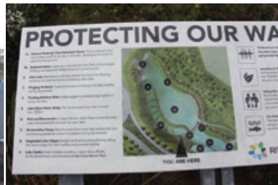
Signage displaying the elements of a constructed wetland designed to reduce run-off, improve water quality and assist in flood mitigation, Riverstone Rise Estate, Boyne Island.
