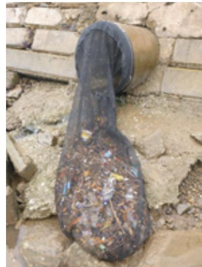
Image of point source debris sampling trap over a central Gladstone stormwater drain outflow. This debris was captured after rainfall of approximately 50 mm. (Image courtesy CQUniversity Gladstone Environmental Centre)
