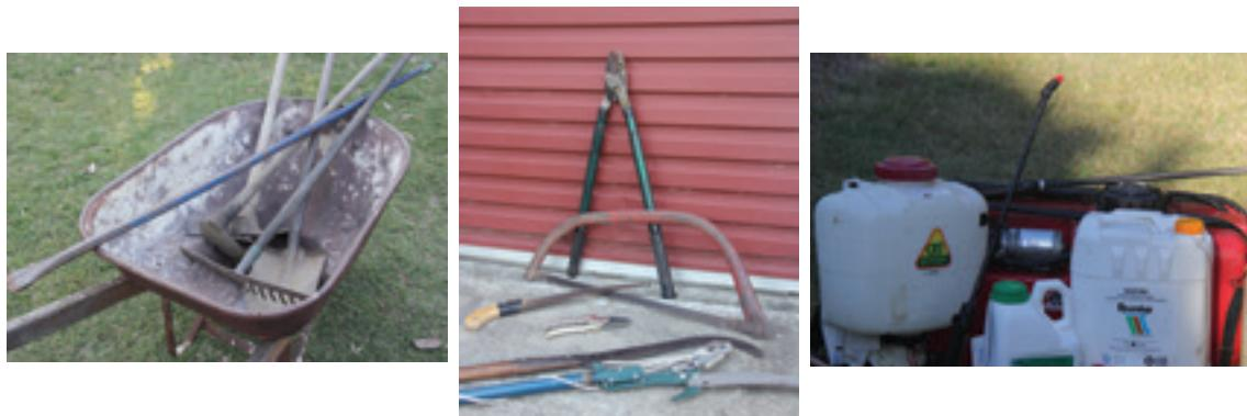
Images of weed removal tools. Left: a range of cutting tools used for weed control. Middle: a range of digging tools used for grubbing weeds. Right: a range of chemical application equipment and herbicides available for weed control works.
