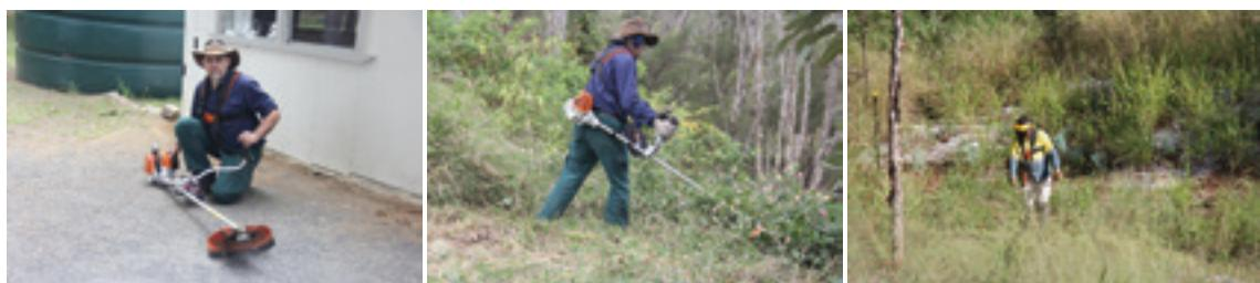
Images of brushcutting. Left: Brushcutter with blade attachment for cutting heavy vegetation. Centre: Using a brushcutter to cut access into a lantana thicket. Right: Brushcutting to control weeds around a revegetation site, Western Basin haul road. Note: operator wears safety equipment.
