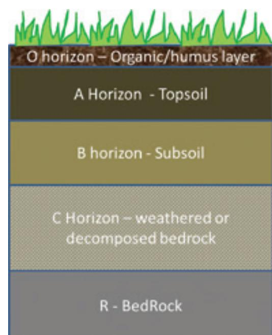
Soil profile diagram. Generally Australian soils have a thin organic (O) layer and thin topsoil layer (A Horizon).
