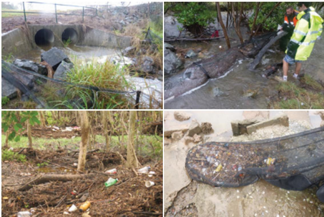
Images of stormwater drains and debris. Top left: Urban drain in flood. Top right: CQUniversity researchers check a stormwater debris monitoring net. Bottom left: Debris accumulates in a creek system after a flow event. Bottom right: A stormwater debris net traps a large amount of litter, in central Gladstone. (Top left, top right and bottom right images courtesy CQUniversity, Gladstone Environmental Centre. Bottom left image courtesy Conservation Volunteers Australia, Gladstone).
