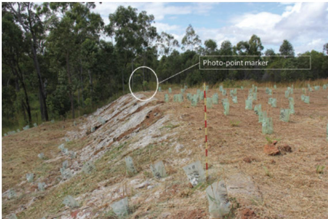
Labelled image of a photo taken at a photo monitoring site, Western Basin haul road, Gladstone (note the graduated pole used for scale).
