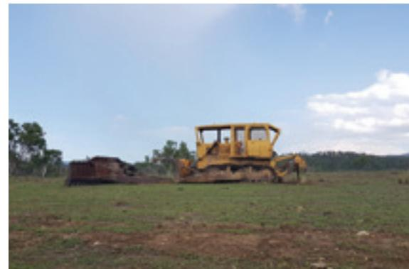
Image of a dozer fitted with rake that could be used to mechanically remove weeds from a large area.
